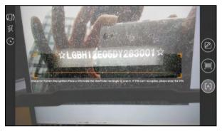
Place the VIN inside the viewfinder rectangle to scan it. The most recognizable location for this number is in the top left corner on the vehicle's dashboard. Other locations include the driver's door or post, and the firewall under the hood.
