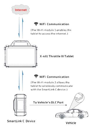
If the SmartLink device is successfully activated, it will be automatically bound to the tablet. In this case it is not necessary for the user to manually configure it again.
